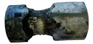
With every compression cycle, energy is pumped into the elastomer material. Unless the roller covering is formulated to be extremely elastic, a large portion of this energy will be stored as heat – the roller gets hotter and hotter, thereby increasing the danger of dynamic blow-out.
