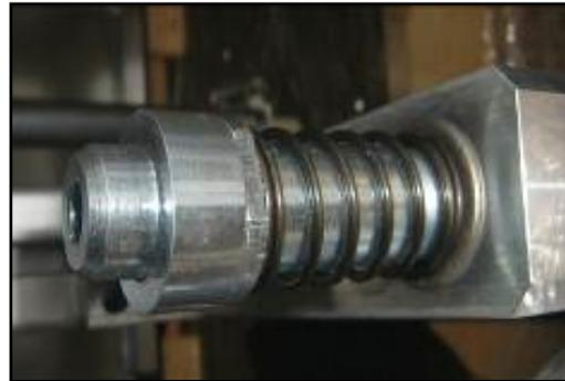
1 Drive spindle → pivot center for Heidelberg (for other presses pivot center is different)
