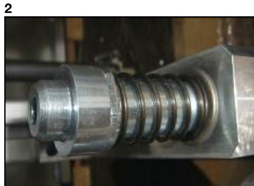
1 Drive spindle → pivot center for Heidelberg (for other presses pivot center is different)
